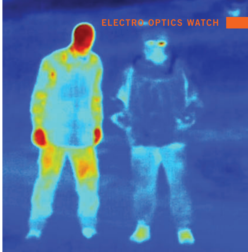
▲ The Army is surveying industry for suppliers of special camouflage fabric to help warfighters conceal themselves from infrared sensors.
