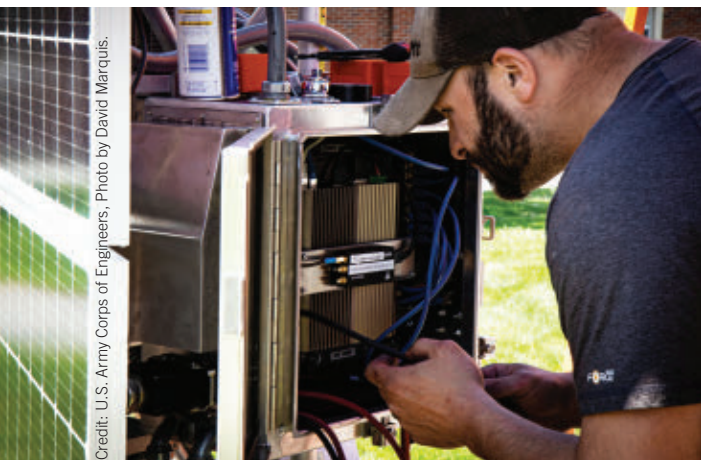
▲ Technicians assemble a newly engineered automated terrestrial laser scanning system (A-TLS) on a 12-foot-tall tower affixed with multiple lidar laser scanners, meteorological sensors, and solar panels to map where components go prior to the tower being disassembled and shipped to Alaska.
